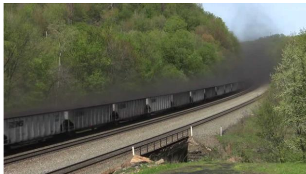
Figure 1.1 - Removal of dust from gondola cars during coal transportation ( https://images.app.goo.gl/fPdPY1FJt3Gushxm7 )
