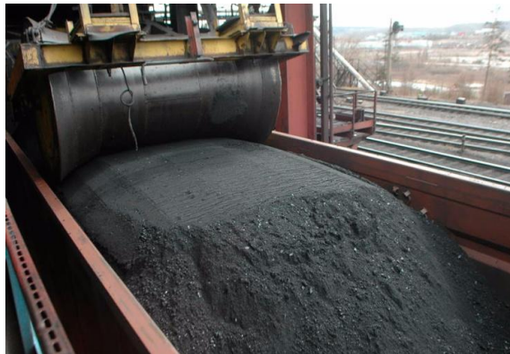
Figure 1.7 - The use of a special roller for leveling and compacting the surface of the load
