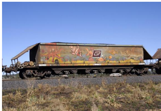
Figure 1.11 - Application of inclined plates in a gondola car (Australia)
