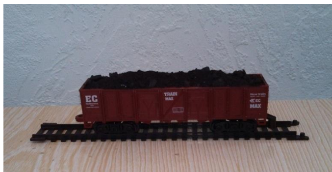
Figure 4.4 – Model of a wagon with coal (loading with a «cap»)
