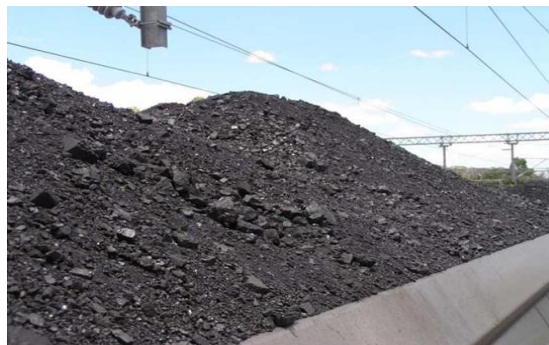
Figure 4.3 – «Cap» of the cargo exceeds the height of the board of the wagon [89]
