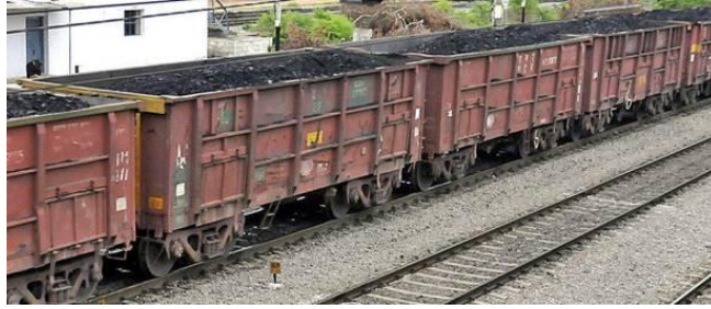
Figure 1.8 - Limit on the height of the "cap" of the cargo ("cap" of the cargo slightly exceeds the height of the board)
