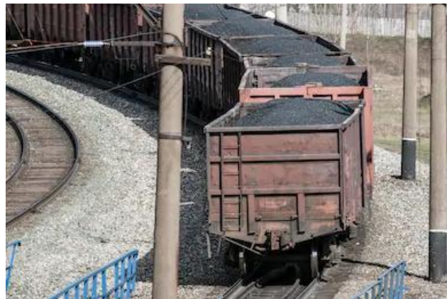
Figure 1.9 - Limit on the height of the "cap" of the cargo ("cap" of the cargo exceeds the height of the sides, but within the recommendations)
