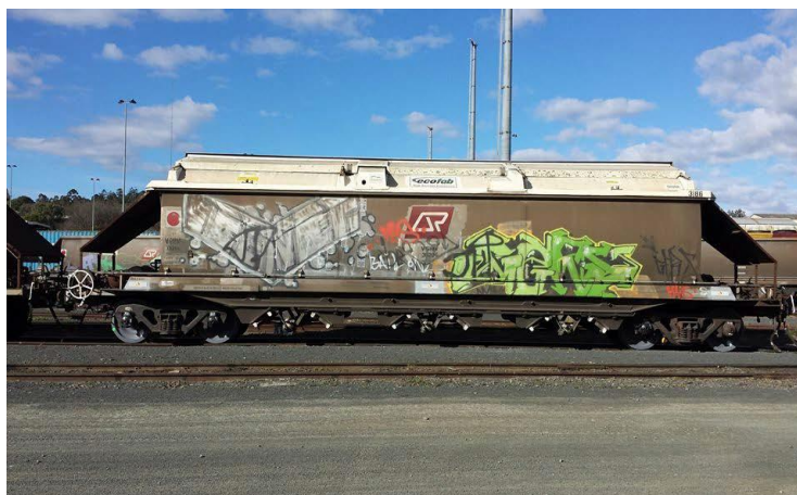
Figure 1.16 - Modernized coal gondola on which the lid is installed, Australia (for comparison, see Figure 1.11) [89]
